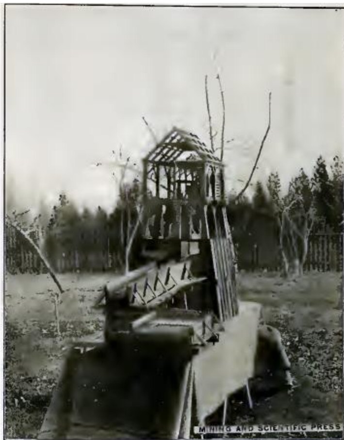
Model of Gravel Washing Plant at Hidden Treasure Mine, Placer County, Cal.
