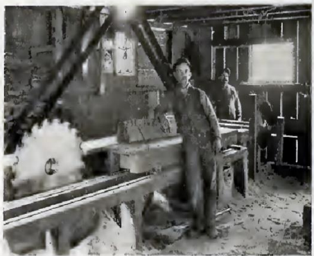
ELECTRICALLY DRIVEN SAWMILL, HIDDEN TREASURE MINE.
